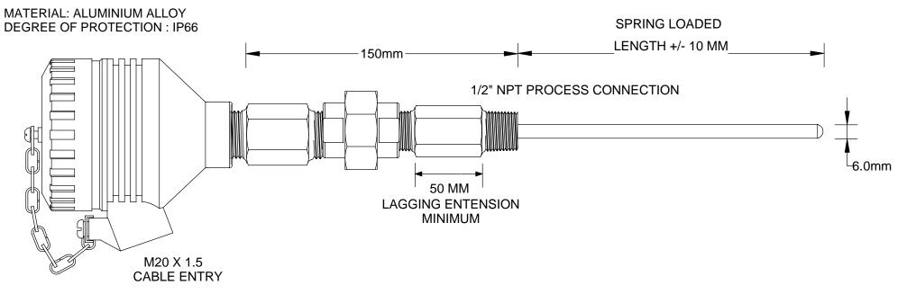
CERTIFIED FOR USE WITH MIMS THERMOCOUPLES AND MIMS RTD SENSORS
